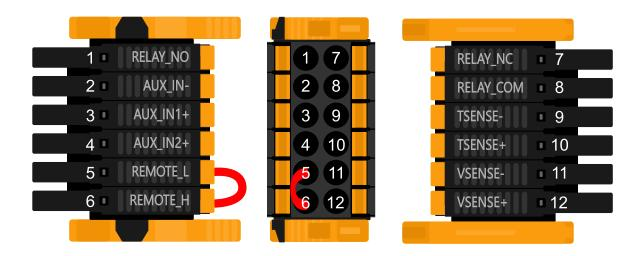
User I/O Connector is located on bottom left side of connection area, diagram shows 3 perspectives. Left Side - Top - Right Side
