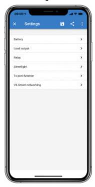
The settings page is accessed by clicking on the Cog icon at the top right of the Home page. The settings page provides access to view or change the settings of the Battery; Load; Streetlight; and Port functions. From this page you can also view Product information such as the Firmware versions installed on the MPPT Solar Charger.
