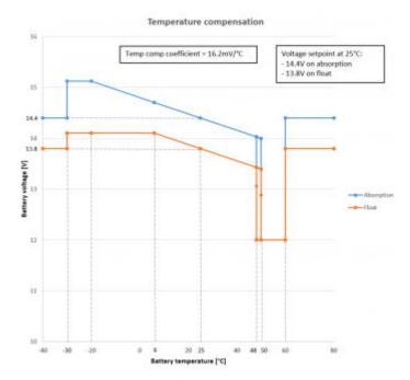
With a temperature sensor installed to the User I/O connection block; the actual battery temperature will be used for compensation; throughout the day.
